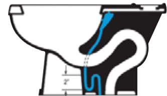
SIDE CUT-A-WAY SHOWING SECONDARY TRAP HT
